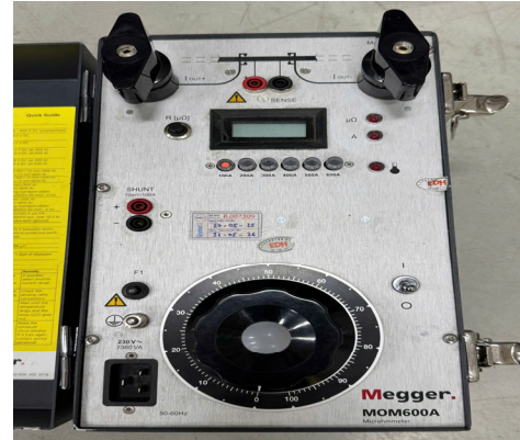
Device for measuring contact resistance MOM 600A
