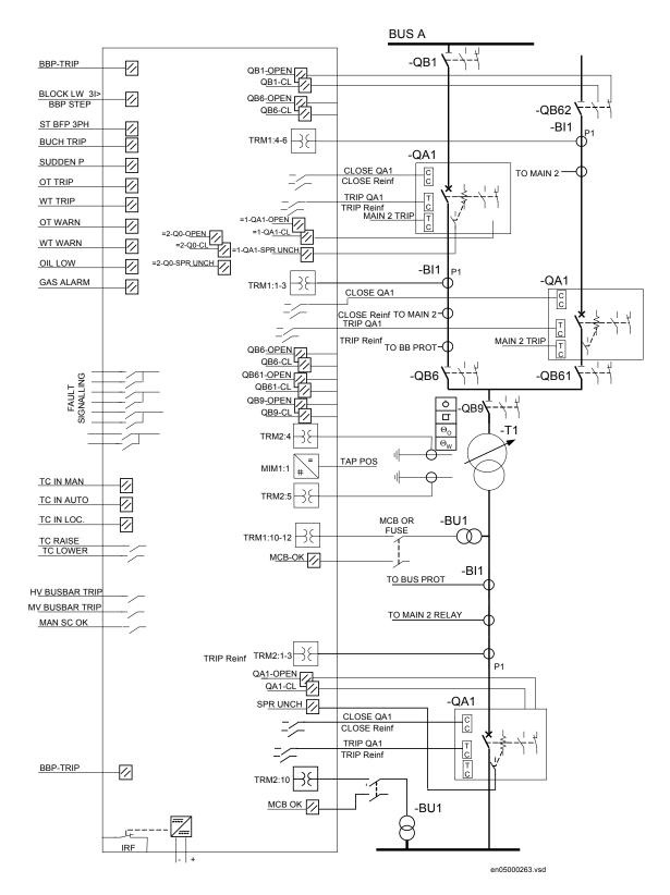
Figure 19. Typical connection diagram for two winding transformer in a multi breaker arrangement. Note! Including IO for control option.
