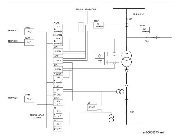
Figure 2. A typical protection application for a two winding transformer in multi breaker arrangements is shown on the figure. The system earthing principle and connection group will vary which gives different detailed arrangements for each application. Breaker failure function is here provided for each breaker.
