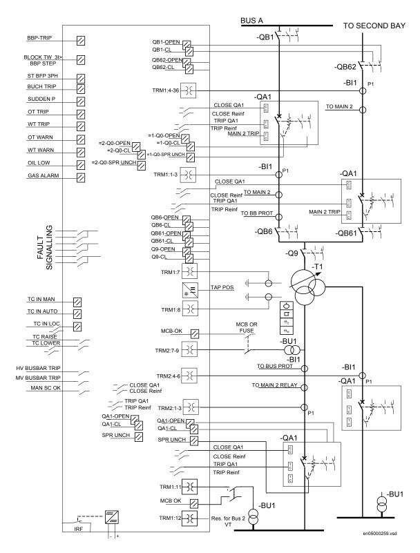
Figure 21. Typical connection diagram for three winding transformer in a multi breaker arrangement. Note! Including IO for control option.
