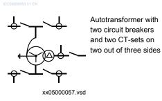
Figure 5. CT group arrangement for differential protection and other protections
