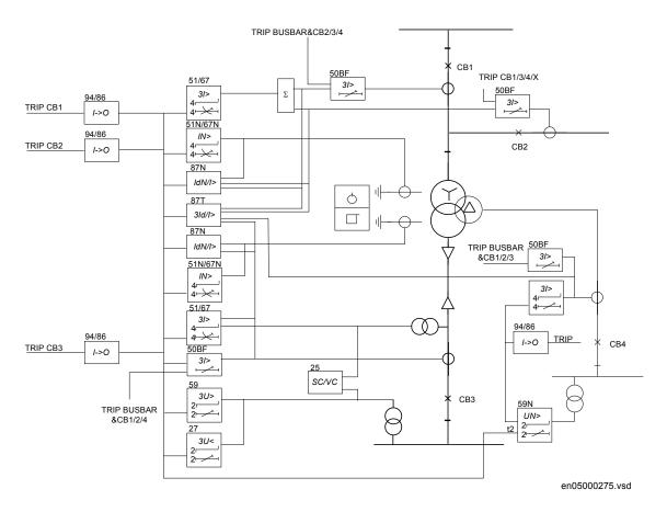
Figure 4. A typical protection application for a three winding transformer in multi breaker arrangements is shown on the figure. The system earthing principle and connection group will vary which gives different detailed arrangements for each application. Breaker failure function is here provided for each breaker.
