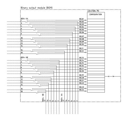
Figure 15. Binary output module (BOM). Output contacts named XA corresponds to rear position X31, X41, and so on, and output contacts named XB to rear position X32, X42, and so on.
