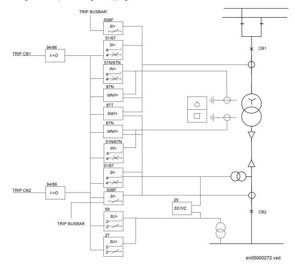
Figure 1. A typical protection application for a two winding transformer in single breaker arrangements is shown on the figure. The system earthing principle and connection group will vary which gives different detailed arrangements for each application.
