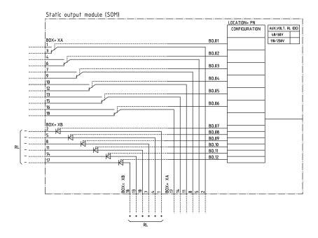
Figure 16. Static output module (SOM)
