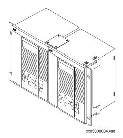
Figure 9. Side-by-side mounting
