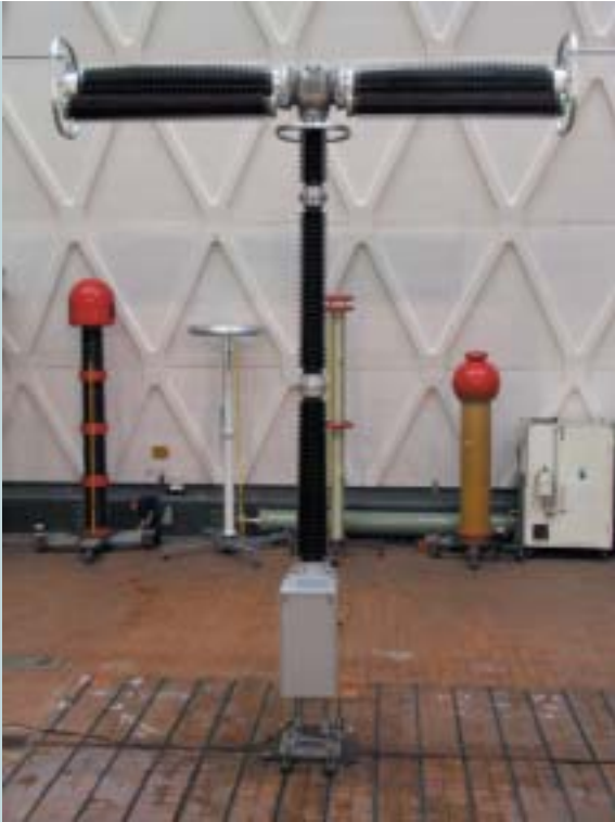
3AP2 FI 550 kV Live-tank circuit breaker at our high-voltage testing laboratory
