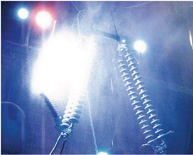
Insulation coordination testing view of the heavy duty EGLA for 275 kV system in wet condition
