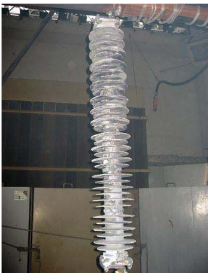
Short circuit testing view of the heavy duty EGLA unit
