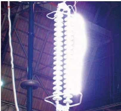
Insulation coordination testing view of the insulators for 275 kV system
